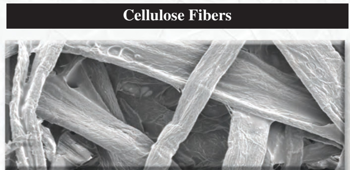
Conventional cellulose fibers are significantly larger than ProTura nanofiber, with larger spaces between fibers. Contaminant loads deep in the media, resulting in higher restriction and shorter service life.
